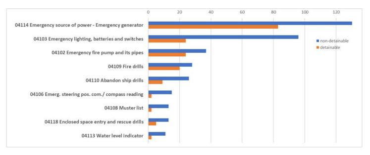
Considering the above deficiencies, we assume the questionnaire items will mainly relate to operational issues and the maintenance of emergency systems like the generator, fire pump and lighting. Furthermore, PSCOs will most likely ask the Master to perform a drill during the CIC. It is still not known if any deficiencies outside the main deficiency group "Emergency Systems", e.g. Machinery Control, will be included in this year's CIC.
